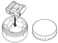
To prevent the print head from drying out, close the lid on the container tightly. If the print head dries out, it will no longer be able to print.
